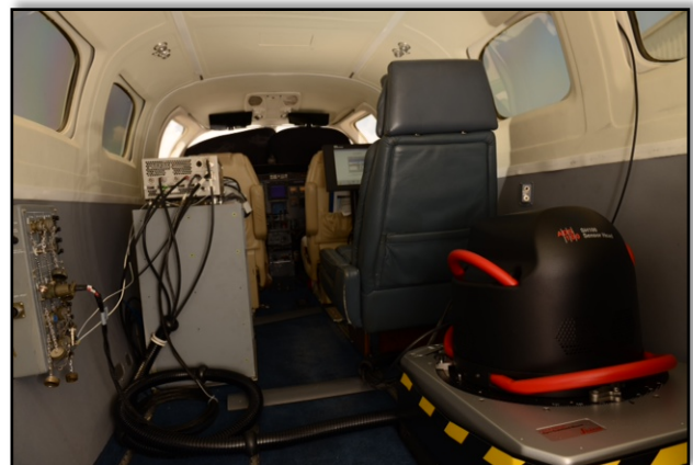
ADS100 Components and Installation in a Surdex Cessna 441 (Conquest) Aircraft.
