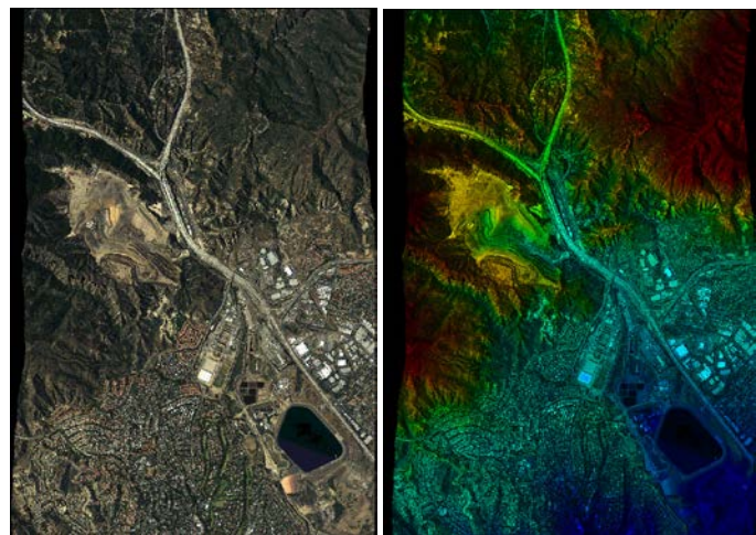
Sample Surdex SGM results with ADS100: image drape (left) and color-coded heights (right).
