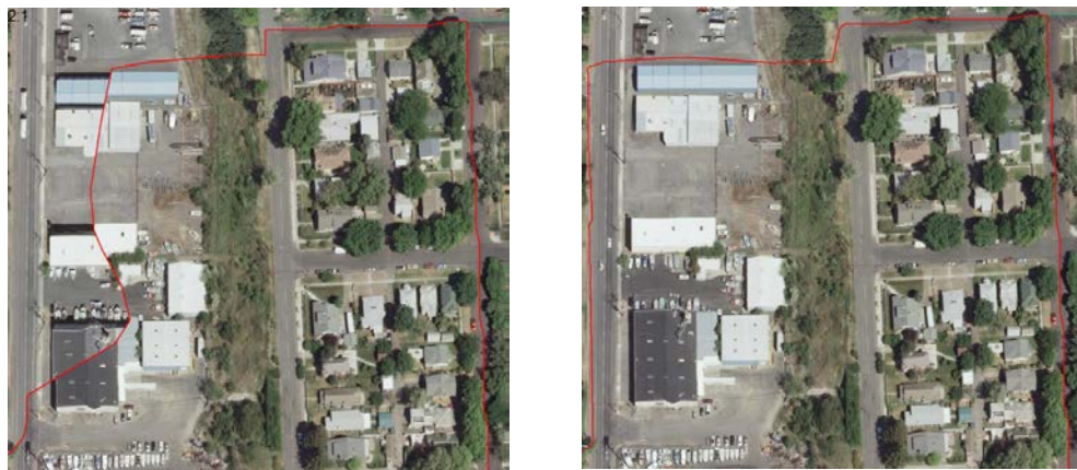
Initial automatic (left) and manually corrected (right) seamlines.
