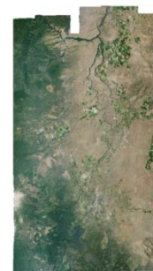
Step 4 Global balance removes residual differences between images
