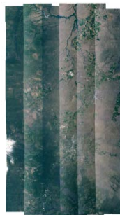
Step 2 Atmospheric correction providing basic color
